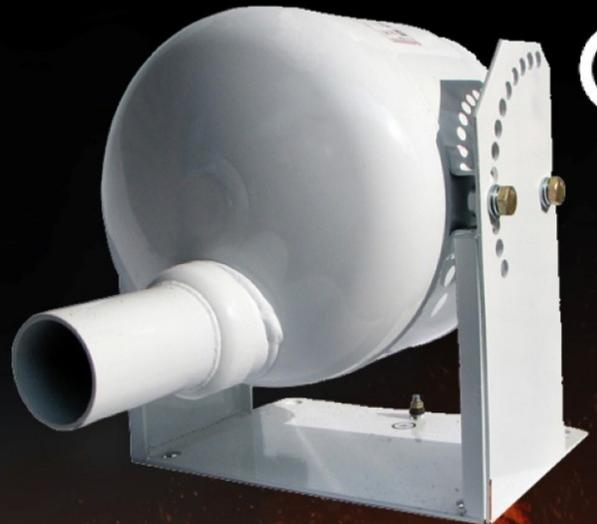
***The module is designed to extinguish hotbeds of ignition in closed cabinets with electronic and electrical equipment of small volume, cable channels, technological equipment on the surface up to 80 m<sup>2</sup> and volume up to 240 m<sup>3</sup>***
